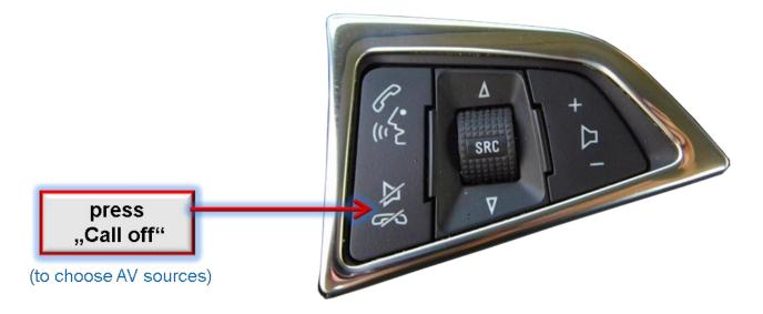
A press of the steering wheel's CALL OFF-button switches the input from factory mode to the inserted video sources. If, by dip switch setting, all inputs are enabled, the order is the following:
